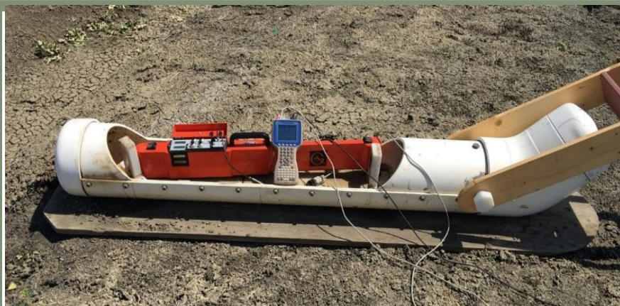
Two transmitter receiver coil separation at 1 m and 0.5 m, for 3 effective depth ranges: 1.5 m and 0.75 m in vertical dipole mode
