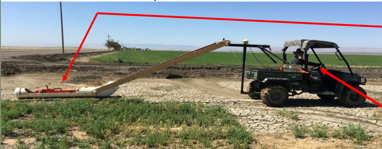
Two transmitter receiver coil separation at 1 m and 0.5 m, for 3 effective depth ranges: 1.5 m and 0.75 m in vertical dipole mode
